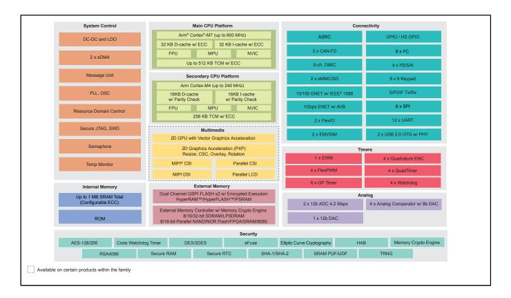
View additional information for i.MX RT1160 Crossover MCU Dual-Core Arm® Cortex®-M7 and Cortex-M4.
