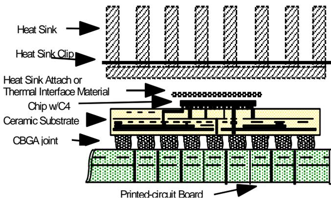
**Figure 2. C4 Ceramic-Ball-Grid Array: Exploded Cross-sectional View with Optional Heat Sink (not to scale).**
