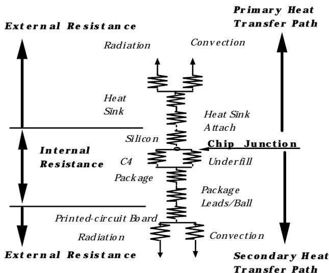
Figure 5. Simplified Thermal Network: a C4-Ceramic-Ball-Grid-Array Package mounted to a Printed-circuit Board. (Note, the internal versus external package resistance.)
