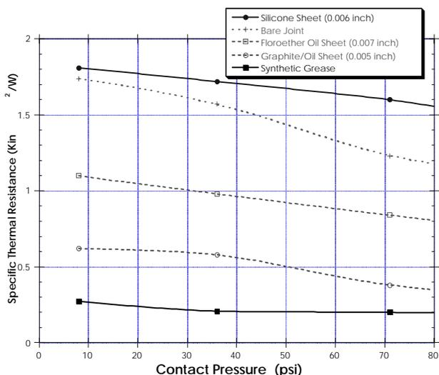
Figure 4. Thermal Performance of Select Thermal Interface Material (adapted from [15])
