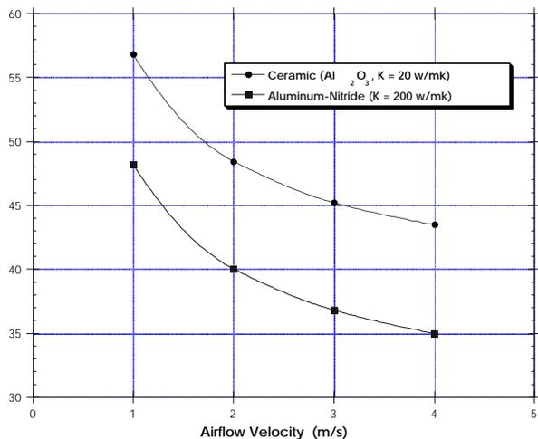
**Figure 8. Model Results for the PowerPC 603 Microprocessor (3 watts) Temperature Rise above the Local Ambient with No Heat Sink for Alumina and Aluminum-Nitride Package Substrate Option.**
