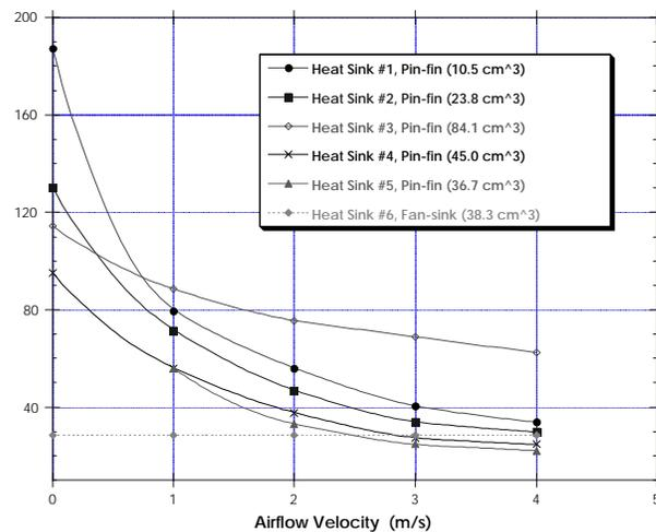
**Figure 9. Model Results for the PowerPC 604 Microprocessor (14 watts) Die-junction temperature Rise for Various Heat Sink Options: Adiabatic Board .**
