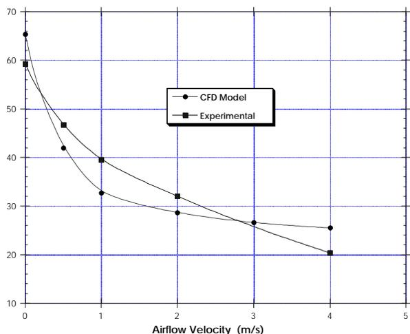
**Figure 6. CFD Model Results versus Experimental Data (3 watt, no heat sink).**
