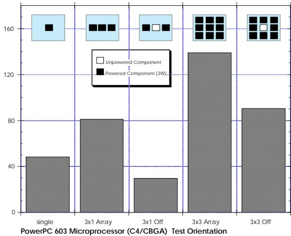
**Figure 10. Model Results for the Populated Board Cases, Interaction Effects of the PowerPC 603 Microprocessor (3 watts) Temperature Rise above the Local Ambient with No Heat Sink.**
