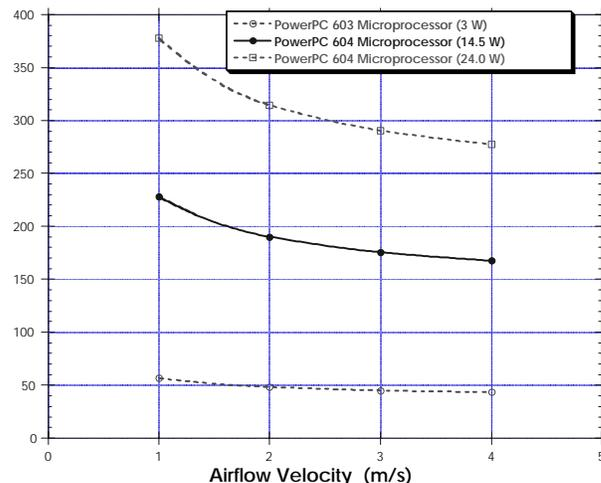
**Figure 7. Model Results for the PowerPC 603 and PowerPC 604 Microprocessor (at 3 and 14.5, 24 watts; respectively) Temperature Rise above the Local Ambient with No Heat Sink.**
